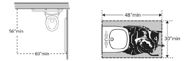
This challenge was overcome by widening the patient restrooms in both rooms. Widening the restrooms created enough space for all of the water fixtures to be placed back-to-back along the same shared wet wall while successfully maintaining ADA compliance. It should be noted that the re- designed restrooms still have a 60" cirlce of clearance to allow for a wheelchair to turn completely around and maneuver.
