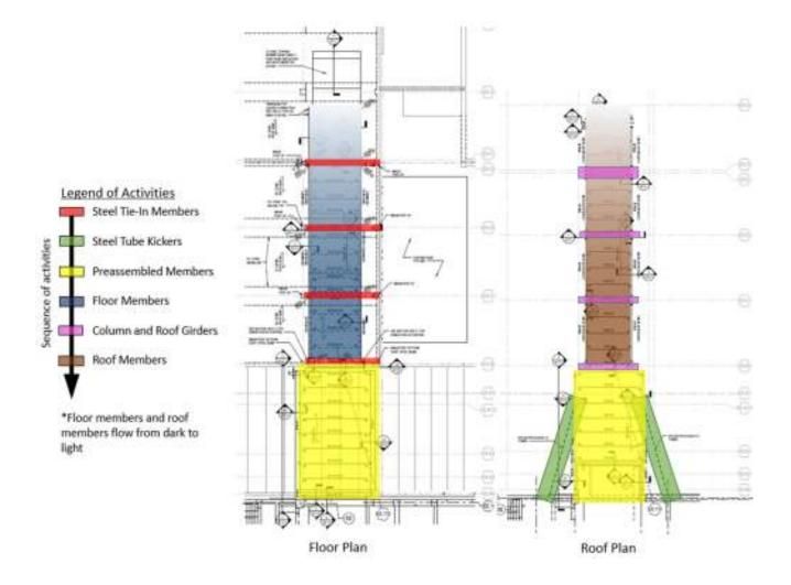
complete by the placing the 3 ¼" lightweight concrete floor. Utilizing the plans from before, a visual representation of the steel installation process can be seen below.
