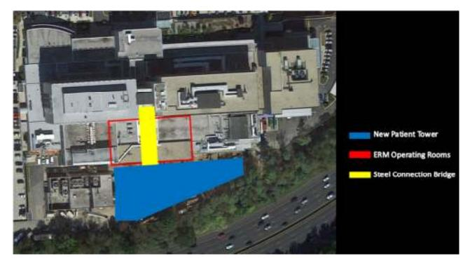
In total this bridge will span 115 feet in length and 16 feet wide for a majority of the bridge. The only portion of the bridge that exceeds 16 feet is the final section connecting to the patient tower. This portion of the bridge, which is 50 feet in length and 23 feet wide, was preassembled by the current project team due to its complex nature and that this section is cantilevering out over the off the patient tower by two
