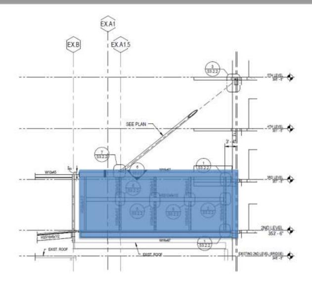
The elevation above provides a great look at how there is no existing column located in the already existing facility it is being built capable of supporting this section's load.
