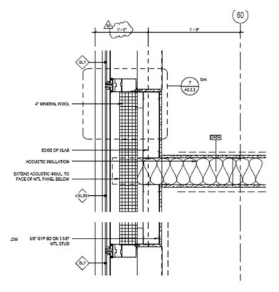
structure behind giving the building a continuous glimmer in the sun. Between the spandrels glazing and structure 4" of mineral wool insulation with an aluminum foil faced vapor retarder exists providing additional thermal and moisture resistance.
